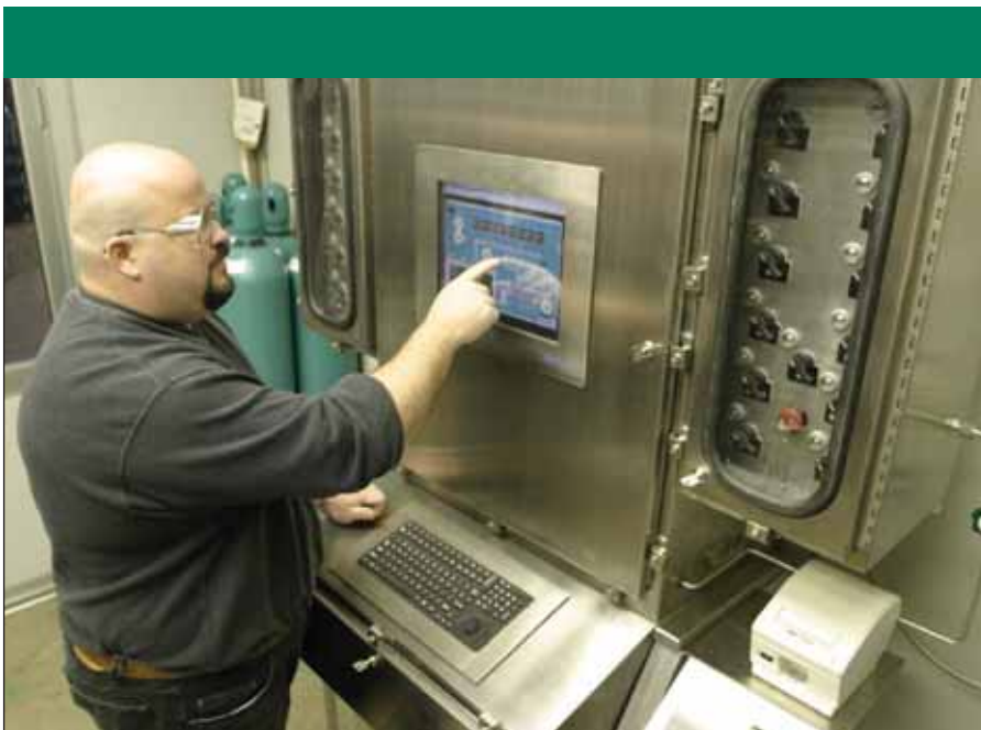
Figure 3: Automated gravimetric blending: Producing a precision mixture using automated gravimetric blending (monitoring the process is Rob Shock of Airgas, Cheshire, Connecticut, pictured above).
