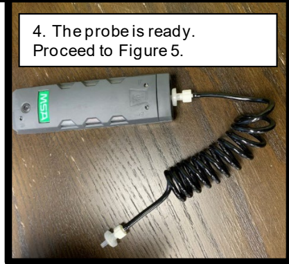
Figure 4 – Preparing the Pump Probe
