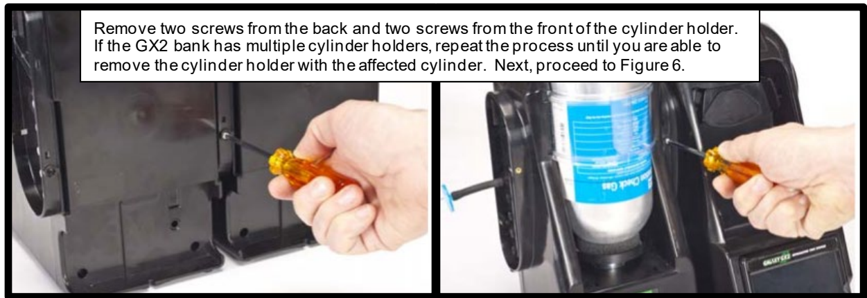
Figure 5 – Removing a Cylinder Holder from a GX2 Bank
