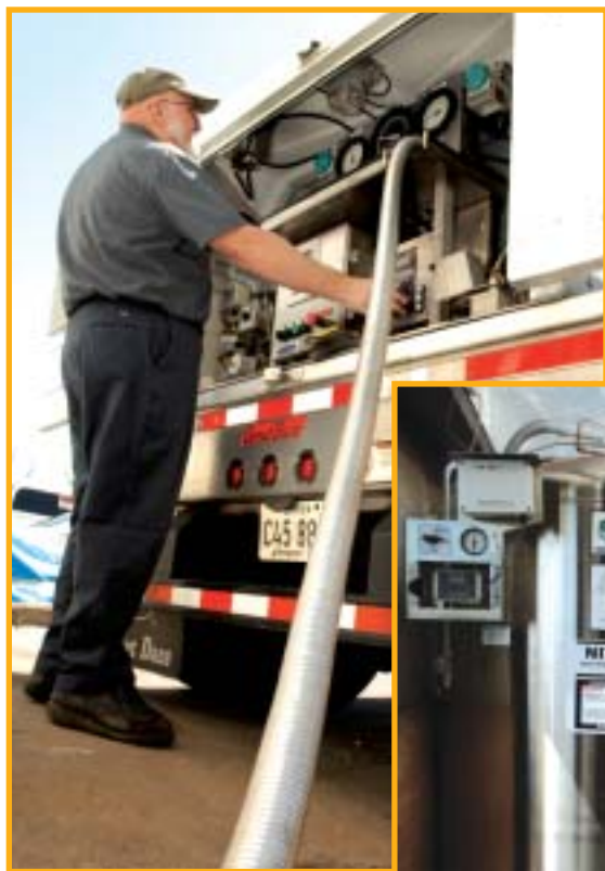
Airgas driver, Kenneth Alexander, refills Cutting Edge Laser's microbulk tank (left) and adjusts the VHP Perma-Cyl below. The truck maintains pressures between 420-450 PSI during refills, helping to reduce downtime.
