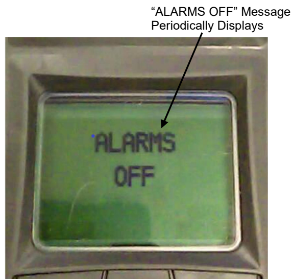
Figure 2: Monochrome Display Showing Alarms Disabled
