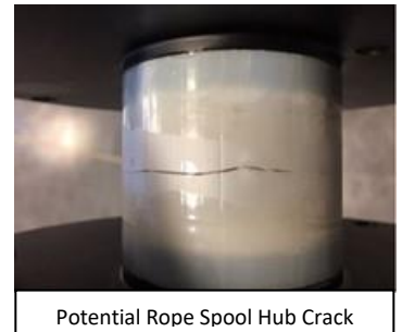
Potential Rope Spool Hub Crack
