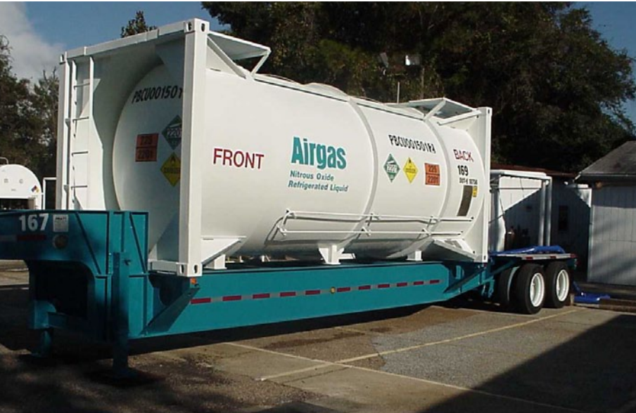
An Airgas bulk tank used to store refrigerated nitrous oxide (N 2 O)
