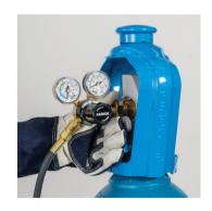
3 Open lever 1 (orange) for partial flow and both levers for full flow
