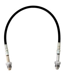
**Description:** These flexible pigtails are for general- or industrial-purpose use. The pigtails consists of a 30" nylon Synflex hose, a brass nickel plated check valve CGA on the cylinder end and a standard CGA on the other end.
