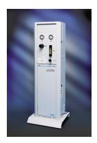
**Description:** The Airgas® Y80-N214 and Y80-N222 Membrane Nitrogen Gas Generators produce up to 72 slpm of compressed nitrogen on-site. The purity level of the nitrogen is defined by the user for the application and may range from 95% to 99.95%. The generator can also be used for solvent evaporation as well as supplying dry nitrogen to analytical instruments.
