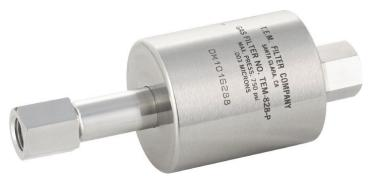
**Description:** The LF410 and LF420 Series in-line gas filters are designed specifically to remove sub-micronsize particulates from process gases. They provide guaranteed 0.003-micron, absolute filtration efficiency and long service. Unlike other gas line filters, the LF410 and LF420 Series filters will not shed particles. The 316L stainless steel housing withstands high operating pressures and provides maximum safety and application compatibility.
