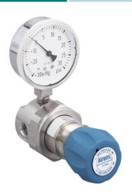
**Description:** This absolute pressure regulator is capable of accepting a line pressure of atmospheric to 250 psig and reducing it to within sub-atmospheric to 10 psig. This regulator is designed for high-purity gas systems and systems which handle highly corrosive media. Only Hastelloy C-22 and PTFE material are in contact with the flow media.
