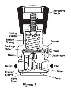
the diaphragm, which pushes the valve stem open. This releases gas into the low-pressure chamber, exerting an opposing force on the diaphragm. An equilibrium is reached when the spring force on the diaphragm is equal to the opposing force of the gas in the low-pressure chamber.
