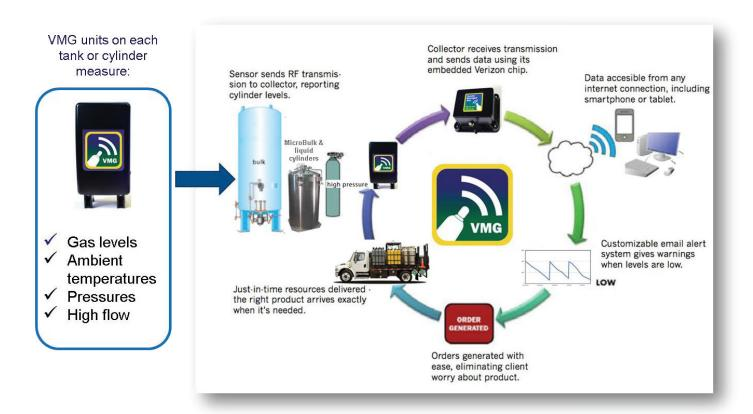
**Description:** Airgas and Vendor Managed Gas have partner to provide a low cost monitoring program for cylinder and bulk applications. A complete system can be preconfigured and installed on our regulators and change over manifolds before they are shipped. This allows for easy start up and instantly providing you information on your gas usage, and eliminates any worries or hassles of running out of gas to your applications, as well not having to install the readers and create the network.
