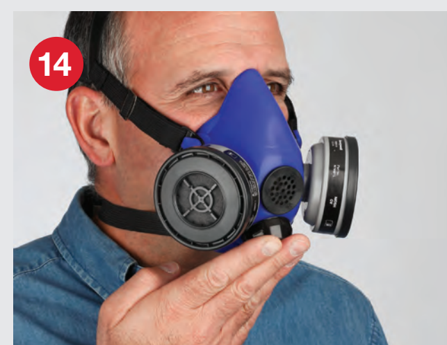
Positive Pressure Seal Check: Place the palm of your hand over the exhalation valve so it is completely sealed and exhale gently. If you have a good seal, the facepiece will be pushed away from your face very slightly.
