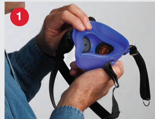
Check the facepiece to make sure it is in good condition, without any holes or tears. Check the cartridge connectors to make sure they are not cracked and are fully inserted into the mask.
