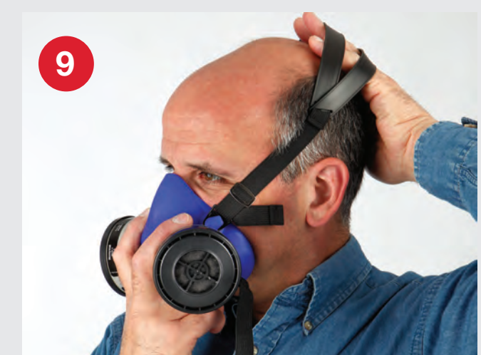
With your other hand, position the plastic straps so they are centered on your head. Remove any slack in the upper straps by pulling the two end tabs back and toward your ears. DO NOT TIGHTEN AT THIS TIME.
