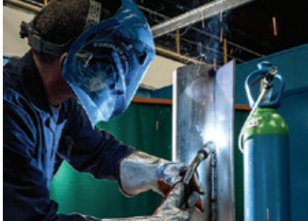
MIG welding of stainless steel
