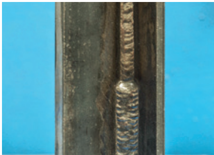
Multi pass welding – vertical up
