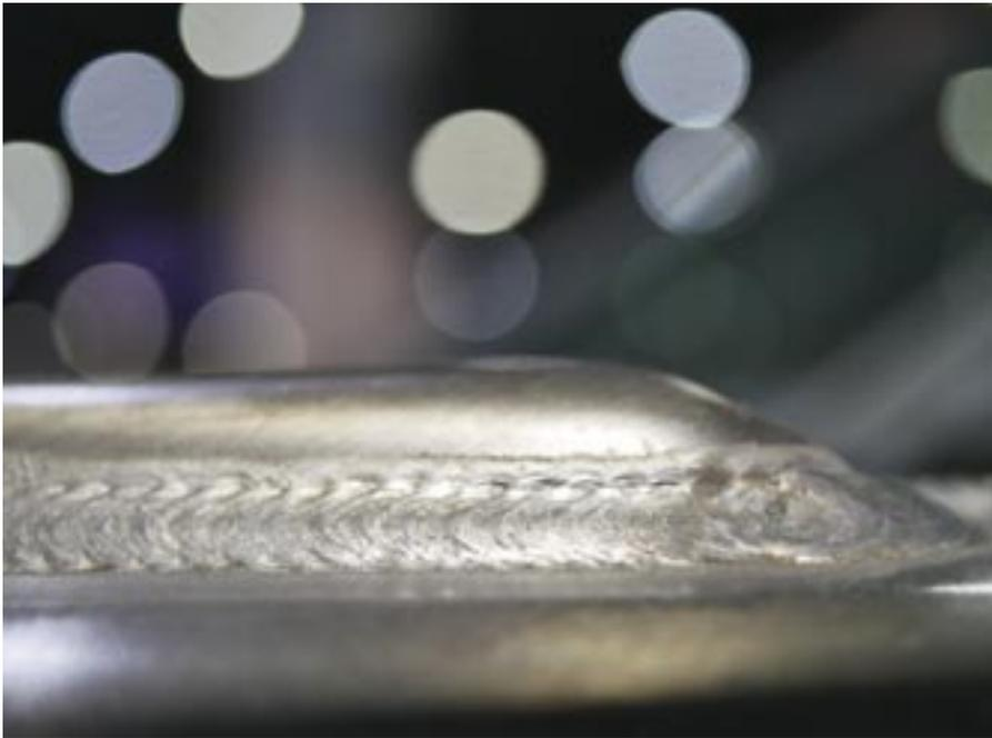
**Fig. 2 — Welding thicker or heavier aluminum sections requires a high heat input to satisfactorily join the metal.**
