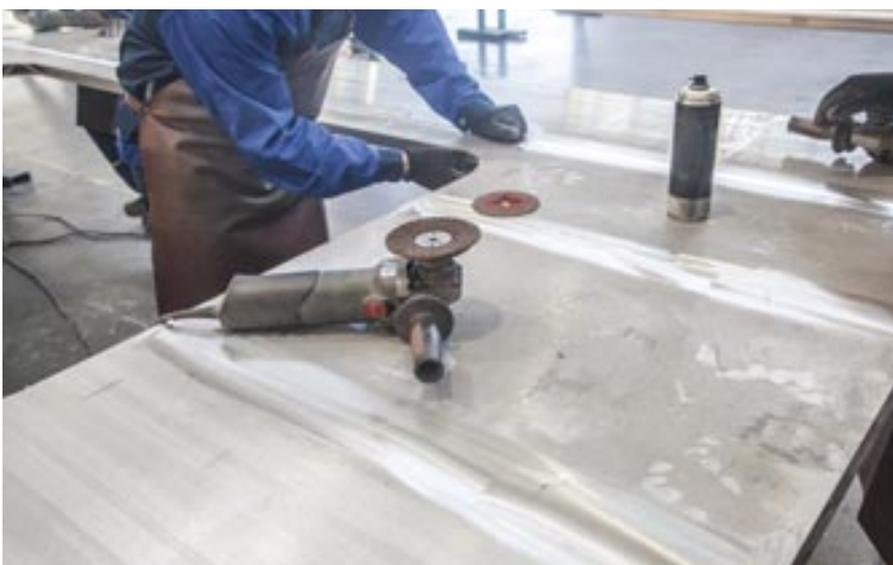
**Fig. 3 — When welding aluminum, it is necessary to remove as much oxide as possible to allow the arc to deliver its heat to the weldment properly. This can be done with scraping, grinding, or brushing, but care must be taken to not embed the oxides deeper into the base metal.**
