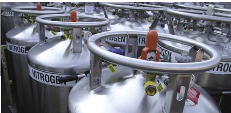
Although liquid cylinders hold their “gas” in liquefied form, the product can be withdrawn from them in liquid or gaseous form
